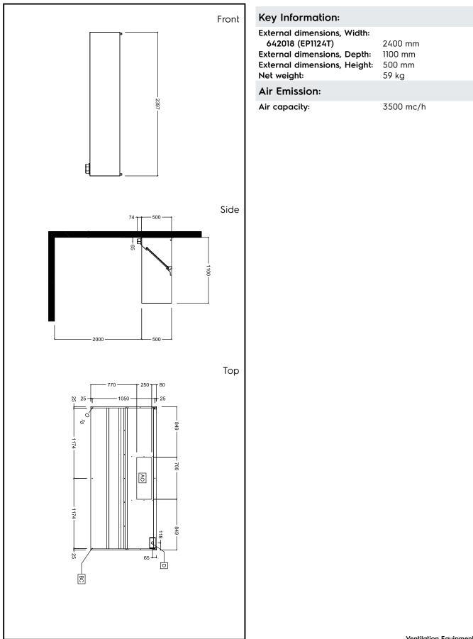
Ventilation Equipment 304 S/S Wall Hood+Filters 2400X1100mm
